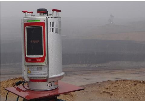
During the course of the monitoring period, moderate rain showers occurred which resulted in some minor slope deformation in a number of locations within the test field. The extents of these deformations was further investigated. However, as there were a number of smaller events, only the most pronounced were investigated. Typical deformations were selected to provide a representative sample of the overall performance for each system.
