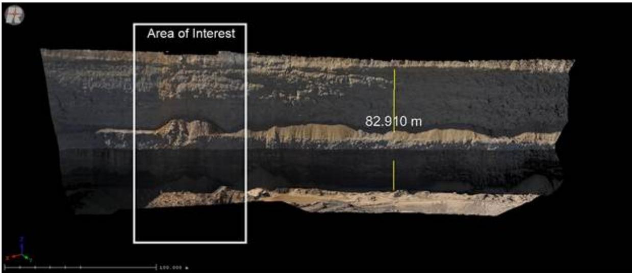
Figure 4. Coal mine high wall mesh colorized by close range photogrammetry (RGB) from Nikon D700.
