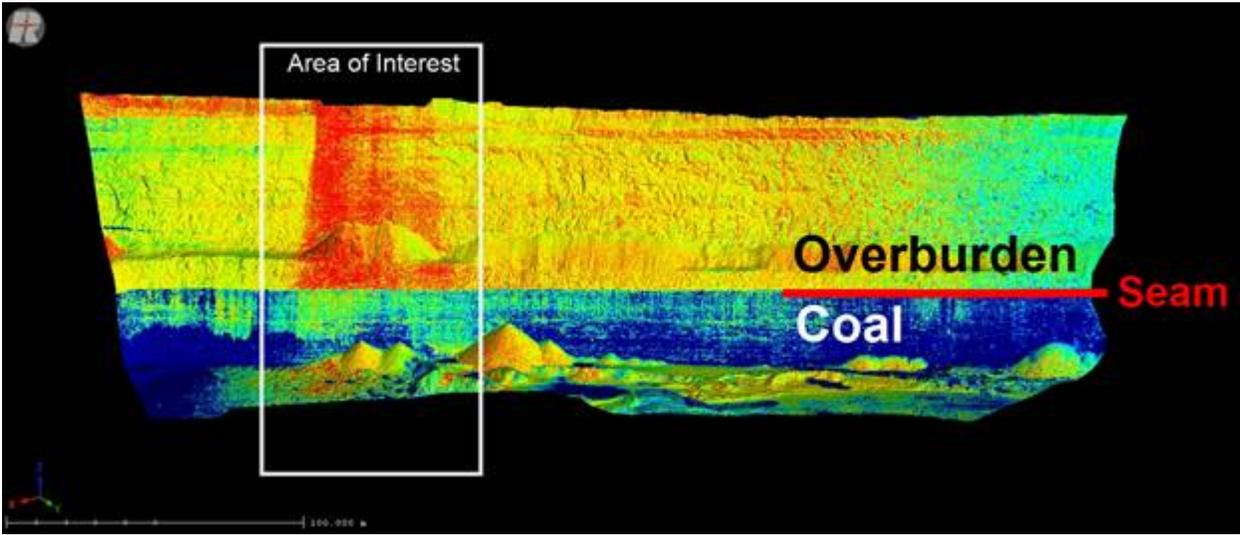
Figure 5. Coal mine high wall mesh colorized by relative reflectance from *Riegl VZ-400* at a range of 160m.
