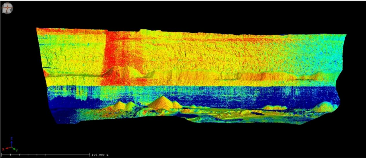
**Figure 8. Coal mine high wall colored by reflectance**
