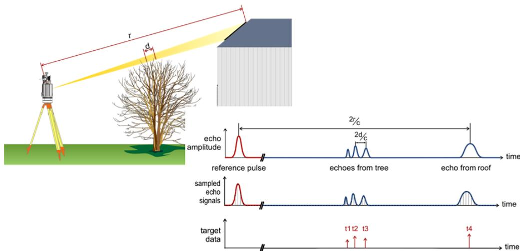
Figure 3. Online waveform single pulse explanation diagram
